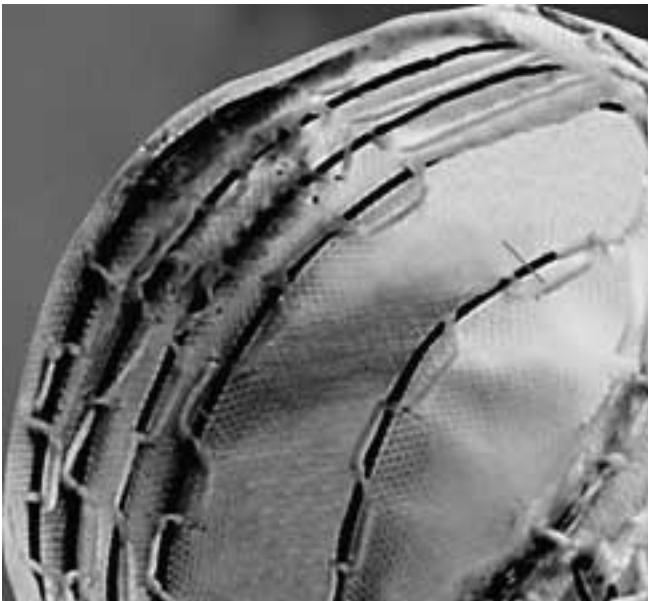
Figure 1.—Proximal stent-graft demonstrating orientation of nitinol wire on polyester graft.
